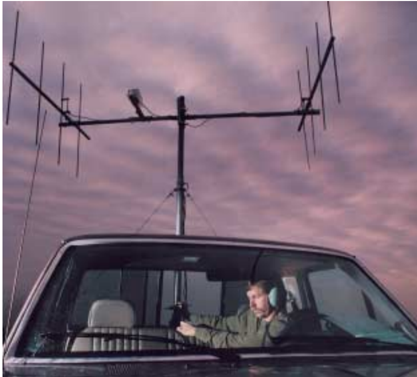
Figure 2. Robert Wagner operating truck-mounted twin yagi antenna system with electronic compass engine used to track black bears in south central Louisiana (1995–96).
