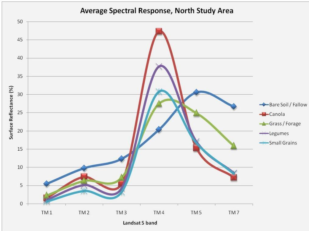
Figure 2.6: Spectral values (in surface reflectance) of the different classes in the main Landsat TM bands for the North study area.
