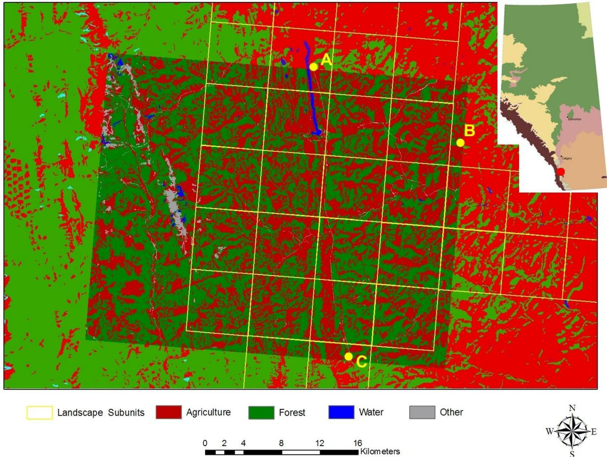
*Figure 3.2: Shows correlation between a classified IRS image (darker colored square in center) and the FMF land cover map (lighter colors), after combining the Landsat classes to match those used in the IRS image classification. Points A, B, and C are located at areas that showcase how the two images are in thematic agreement.*
