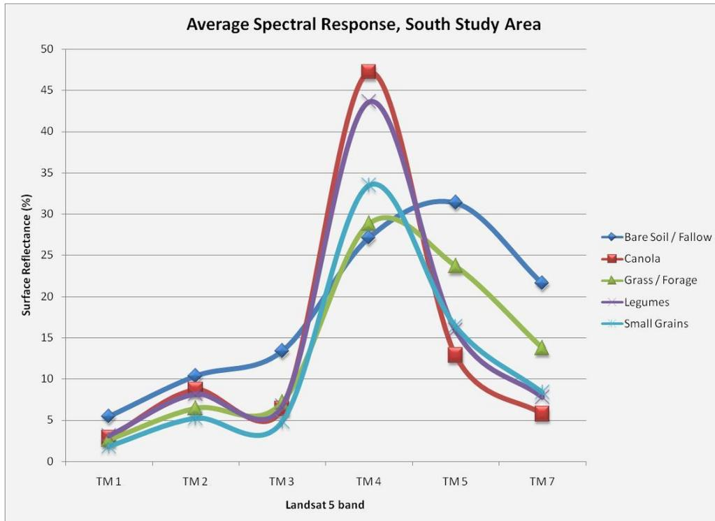
Figure 2.5: Spectral values (in surface reflectance) of the different classes in the main Landsat TM bands for the South study area.
